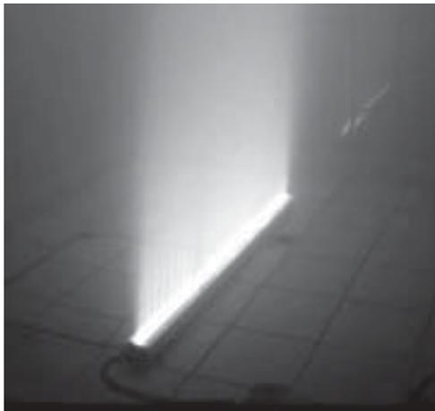
Fig. 4 Near-parallel beam of LED-line
