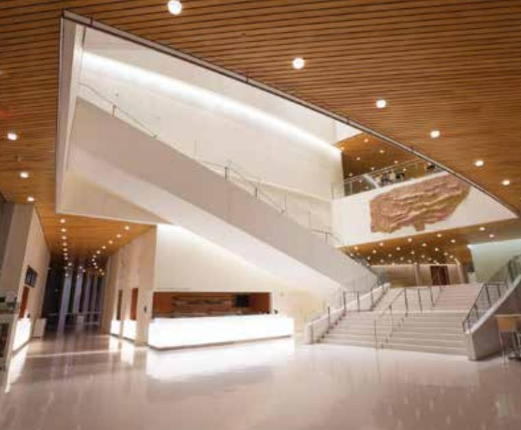
Each is evenly illuminated by one high-output linear fixture, easily accessible through the toe-kick. At the atrium ceiling, cove lighting and custom bracket-mounted fixtures illuminate curving skylights, preserving them as sources of light at night.
