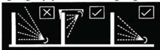
When lighting vertical structures such as advertising signs direct light downwards, wherever possible, to illuminate them not upwards. If there is no alternative to up lighting, then the use of shields, baffles and louvres will help reduce spill light around and over the structure to a minimum.
