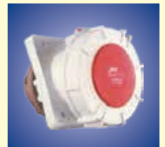
63 Amps Ang. J63 5 AS 3 pole + N + ⊕ IP67
