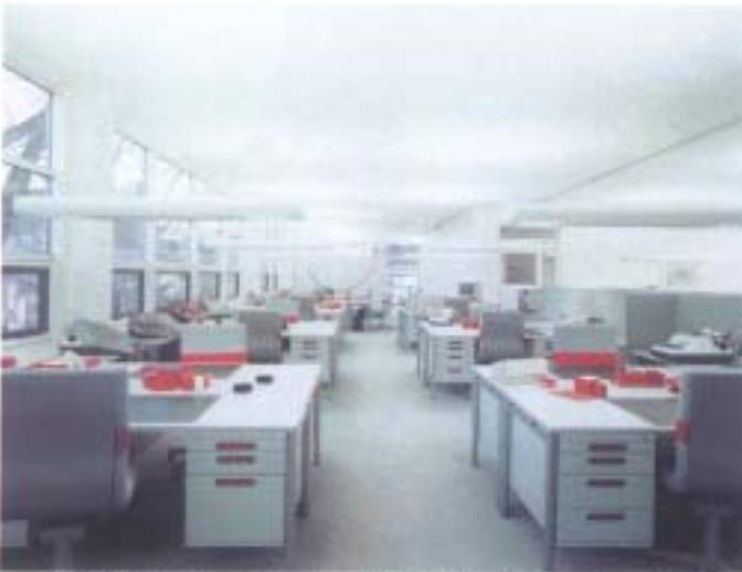
Very 'misty' lighting atmosphere, the proportion of direct light from the suspended luminaires is too low. A new lighting level is created by the suspended luminaires.
