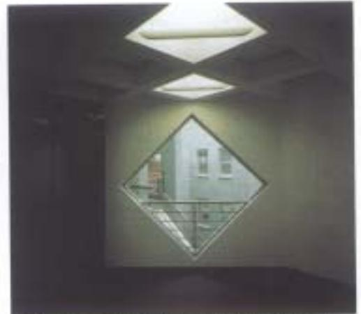
Office lighting details. Finely distributed light in the coffered ceiling and architecture-oriented indirect light and direct light for specific zones.
