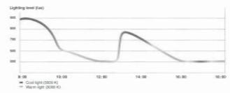
Figure 2. Conceptual lighting algorithm of activity during day time
