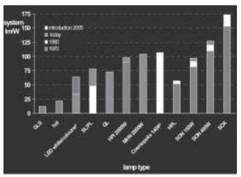
Fig. 3 Luminous efficacy of lamps employed in outdoor lighting (efficacies based on wattages typical for outdoor lighting applications)
