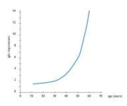
Fig.4 Relation between age and relative amount of light required for reading good print (source:Fortuin [8]).
