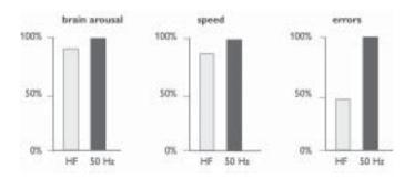
Fig.11 Brain arousal measured as the reciprocal value of the alpha activity of EEGs in persons in offices under 50 Hz and under high-frequency HF (30 kHz) fluorescent lighting. The working speed and errors of a proof-reading task are also given (graph adapted from: Küller and Laike [25]). Subject group:high flicker sensitivity.
