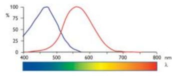
Fig.3 Spectral biological action curve (based on melatonin suppression), in blue, (source: Brainard [7]), and the visual eye sensitivity curve, in red.
