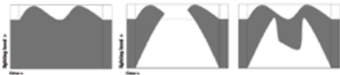
Figure 10: Schematic representation of required artificial lighting for situation with algorithmic lighting (left) and situations shown in figure 9b and figure 9c
