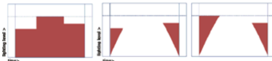
Figure 5: Schematic representation of a control strategies combination 2 a) Evaluation of savings due to use of scenes, compared to all lighting on (installed power based) b) Evaluation of two different scene setting profiles, combined with daylight responsive lighting control. The daylight responsive lighting control is more beneficial in the left picture.
